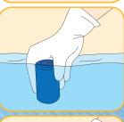
Immerse the roll in the water in a temperature of 20~24 degrees for 3~5 seconds and squeeze 3~4 times in the water for the complete water penetration into the body of the roll.
